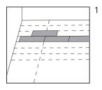
Check the room dimension by measuring or placing the tiles (without gluing) from the middle. Make sure that the widths of the tiles that will be near the wall are identical and greater than 5 cm. If necessary repeat the previous step by drawing new parallel lines to the first ones.
