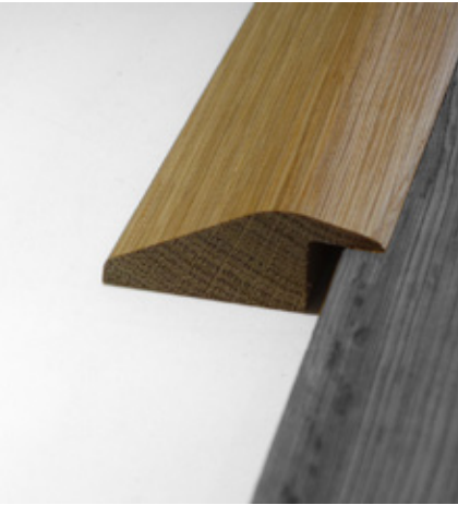
Solid Oak Ramp Edge A solid hardwood profile, fixed to the sub floor which allows for expansion where there is a transition in floor level.
