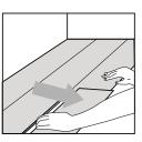
Do not bend connected planks backwards as this will damage it.
