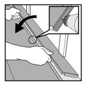
Remove the locking element/hook according to the picture. Use white PVAc glue to connect the planks. Position wedges between the glued plank and the wall.
