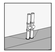
Mark the centre point of the pipes on the plank. Drill holes 20 mm bigger than the pipe's diameter (if gap distance selected is 10 mm). Cut according to the picture. Fix with white glue and replace the floor pieces. Cover the holes with pipe collars or fill with a joint sealer.
