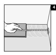
At the end of the first row, put a wedge to the wall and measure the length of the last plank to fit.
