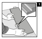
First plank, first row. Start in the left corner with the tongue side facing the wall and the long groove side directly up against the straight edge. Spread enough adhesive to cover one plank width. Use only as much adhesive as can be used during the manufacturer's maximum recommended time for keeping the container open.
