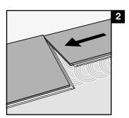
Second plank, first row. Line up the plank gently and tightly to the short end of the previous plank.
