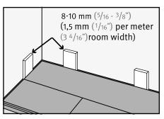
Using the starting wall as reference, snap a chalk line on the subfloor at distance X from the wall as shown in Fig. 1.1. Align the straight edge with the chalk line and secure it to the subfloor.
